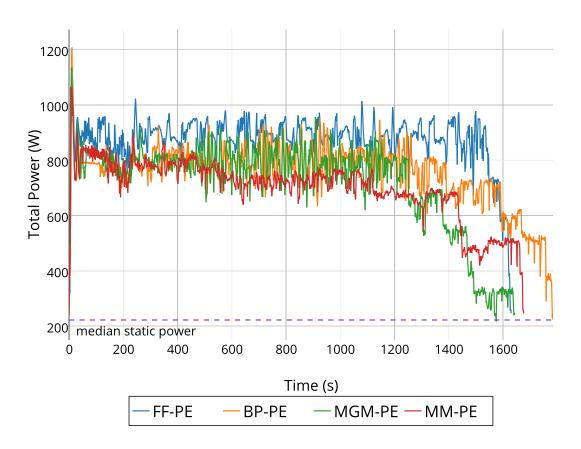
Figure 5.16: Power profile of Heavy Workload run under Progressive Extrema capping.
