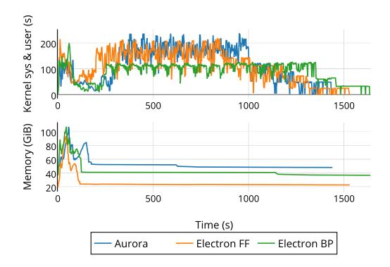
Figure 4.2: Cluster-wide CPU & Memory Utilization of Aurora and Electron without a power cap.
