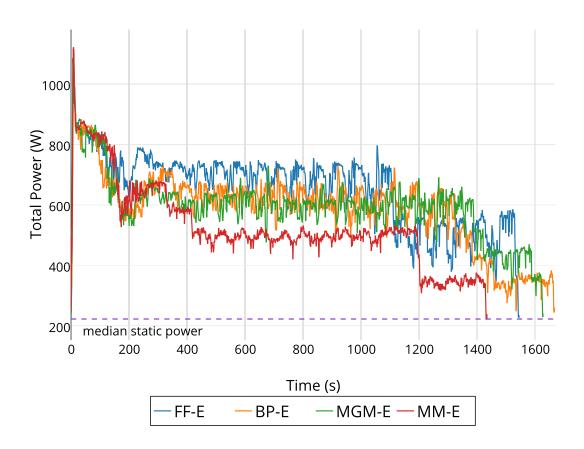
Figure 5.15: Power profile of Moderate Workload run under Progressive Extrema capping.
