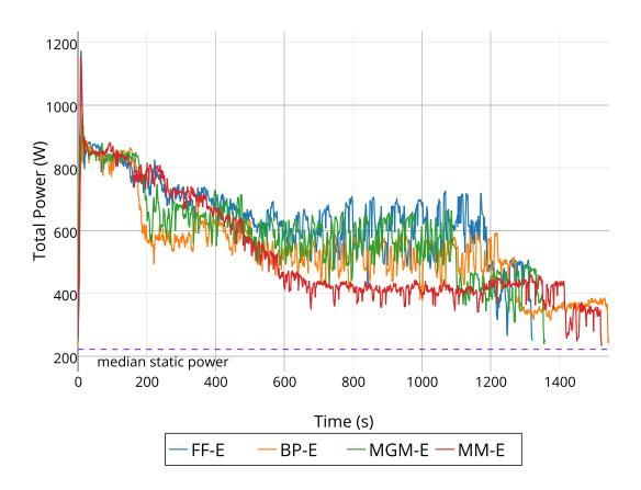
Figure 5.11: Power profile of Light Workload run under Extrema capping.
