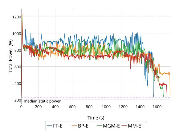
Figure 5.13: Power profile of Heavy Workload run under Extrema capping.
