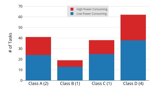
Figure 5.3: Distribution of tasks by classification for a Moderate Power Consuming workload when using Max-Min. The number of nodes for each power class is shown in parentheses. This figure shows Class D bearing a larger burden than the rest of the classes with Max-Min as the scheduling strategy.
