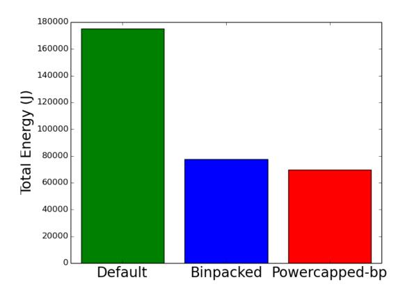
Figure 3.9: Energy Consumption of cluster using MPF-BP.
