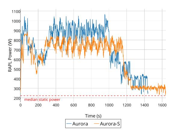
Figure 4.6: Cluster-wide Power Consumption for Aurora and Aurora running under a static power cap.
