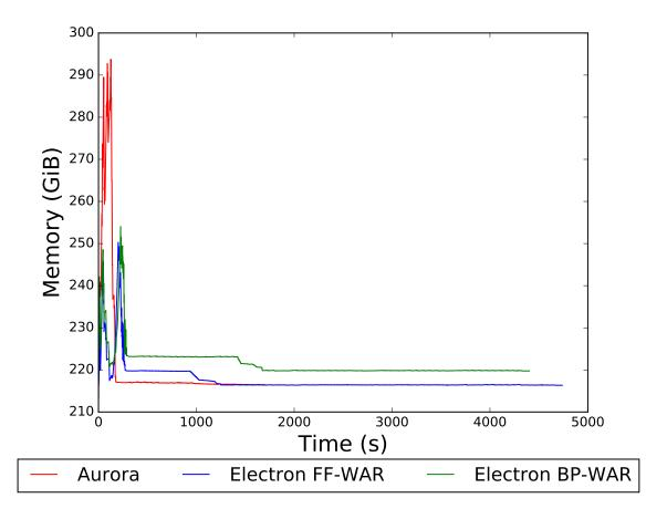
Figure 6.3: Cluster-wide Memory Utilization when WaaR is deployed and the cryptography benchmark is included.
