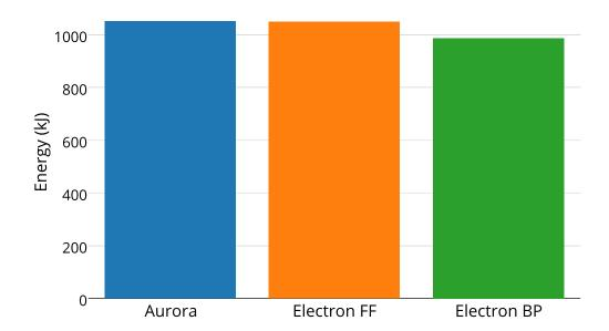
Figure 4.4: Cluster-wide Energy Consumption of Aurora and Electron without a power cap.
