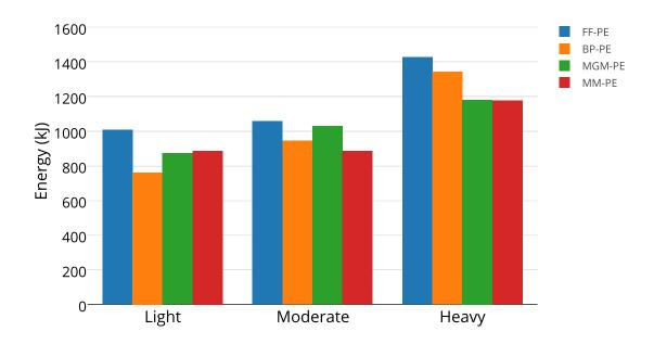
Figure 5.10: Progressive Extrema capped workloads. Comparison of Cluster-wide Energy Consumption for different scheduling policies and classes of workloads in combination with the Progressive Extrema dynamic power capping strategy.
