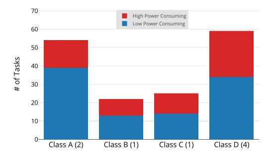
Figure 5.4: Distribution of tasks by classification for a Moderate Power Consuming workload when using Max-GreedyMins. The number of nodes for each power class is shown in parentheses. This figure shows Class A and Class D completing about the same number of tasks in number with Class D processing more power intensive tasks when using a Max-GreedyMins strategy to schedule workloads.
