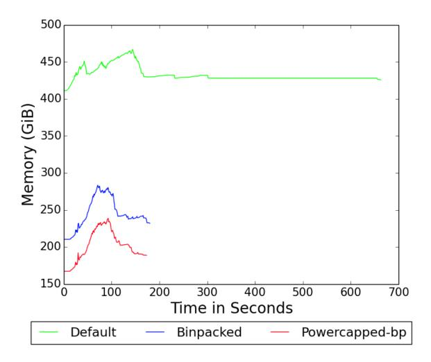
Figure 3.8: Memory Utilization of cluster using MPF-BP.Memory utilization is, at its highest, 147% higher than the bin-packed only run and 157% higher than the power-capped-bin-packed run. The default run expends 77% more energy than the bin-packed only run and 86% more energy than the power-capped-bin-packed run.
