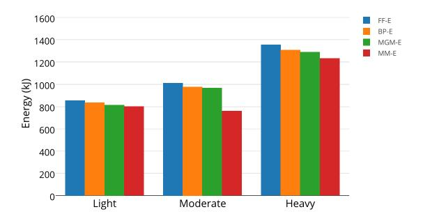
Figure 5.9: Extrema capped workloads. Comparison of Cluster-wide Energy Consumption for different scheduling policies and classes of workloads in combination with the Extrema dynamic power capping strategy.
