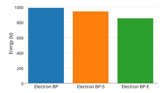
Figure 4.13: Cluster-wide Energy Consumption of uncapped Electron Bin Packed, statically capped Electron Bin Packed and Electron Bin Packed running under Extrema capping.
