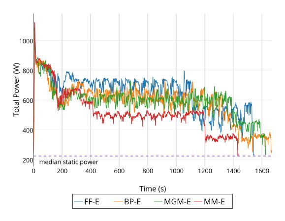
Figure 5.12: Power profile of Moderate Workload run under Extrema capping.
