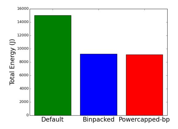
Figure 3.6: Baseline node Energy consumption using MAP. MAP-BP, Baseline Node using the MAP-BP policy. The energy utilization compared to the MPF-BP is 14% higher for the bin-packed-only run and 17% higher for the power-capped-bin-packed run.
