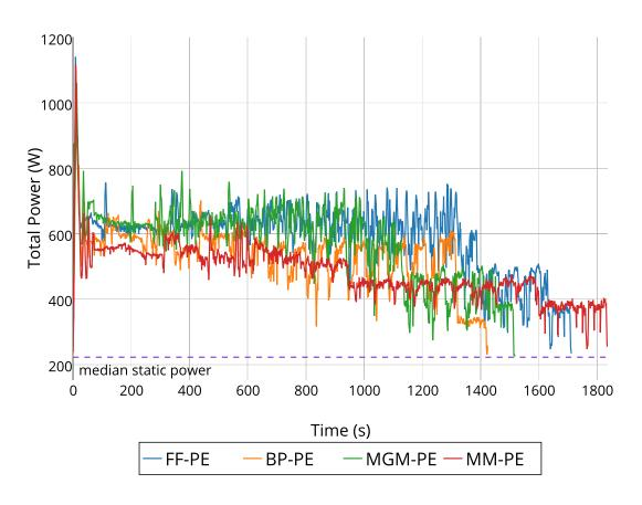
Figure 5.14: Power profile of Light Workload run under Progressive Extrema capping.
