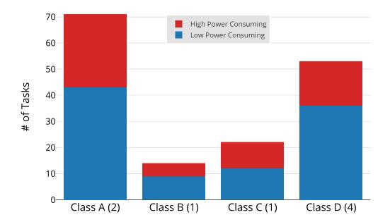
Figure 5.2: Distribution of tasks by classification for a Moderate Power Consuming workload when using Bin-Packing. The number of nodes for each power class is shown in parentheses. This figure shows Class A nodes processing more power intensive tasks than Class D nodes despite having half as many workers when using the Bin-Packing strategy.
