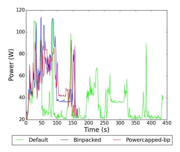
Figure 3.4: Baseline node Power consumption using MAP. The bin-packed only run shows similar power peaks to those observed in Figure 3.1. The most noticeable difference is the decrease in consumption around 100 seconds and a late spike at around 150 seconds. The power-capped-bin-packed run displays similar characteristic with lower peaks by 90% when compared to the baseline and 1% compared to the optimized run.
