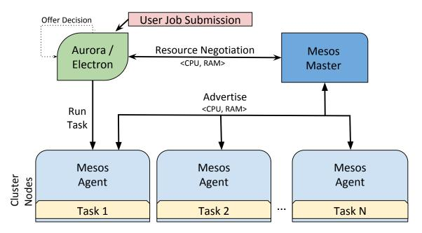
Figure 4.1: Architecture of Mesos and Aurora/Electron. Note that Electron has the same position in the architecture as Aurora.
