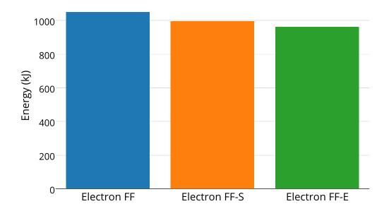
Figure 4.10: Cluster-wide Energy Consumption for Electron First Fit, Electron First Fit running under static cap, and Electron First Fit running under the extrema dynamic cap.
