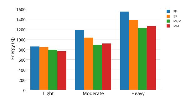
Figure 5.8: Uncapped workloads. Comparison of Cluster-wide Energy Consumption of different scheduling policies when used to schedule different classes of workloads (Light, Moderate and Heavy).
