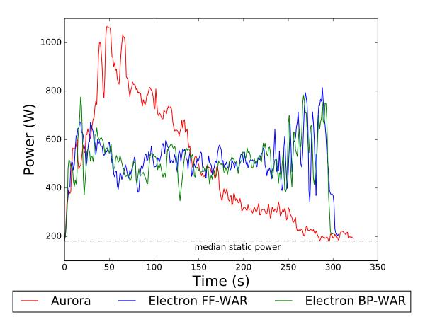
Figure 6.5: Cluster-wide Power Utilization when WaaR is deployed but the cryptography benchmark is not included.
