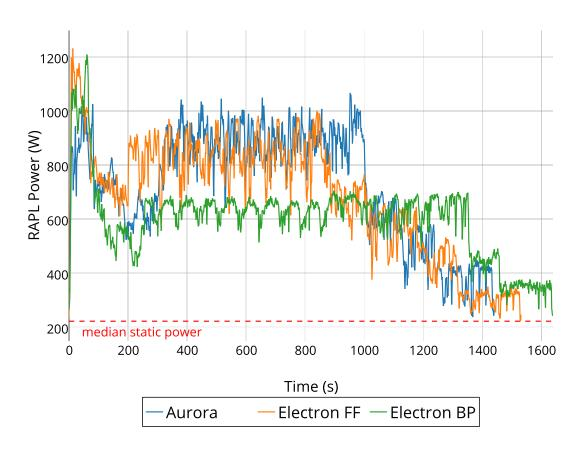
Figure 4.3: Cluster-wide Power Consumption of Aurora and Electron without a power cap.
